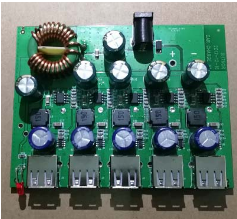
1, independent 5 USB fast charge circuit design
