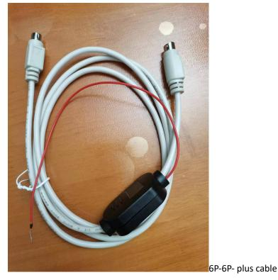
Note: The red power cord is connected to the radio +13.8V power supply.
