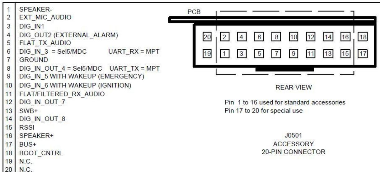
Use "6-pin to 16-pin conversion board" to insert CDM-1250 accessory connector 1-16
