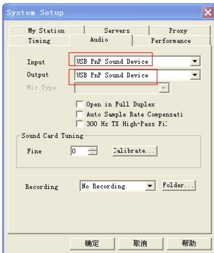
Select audio input and output as: **USB pnp sound device**
